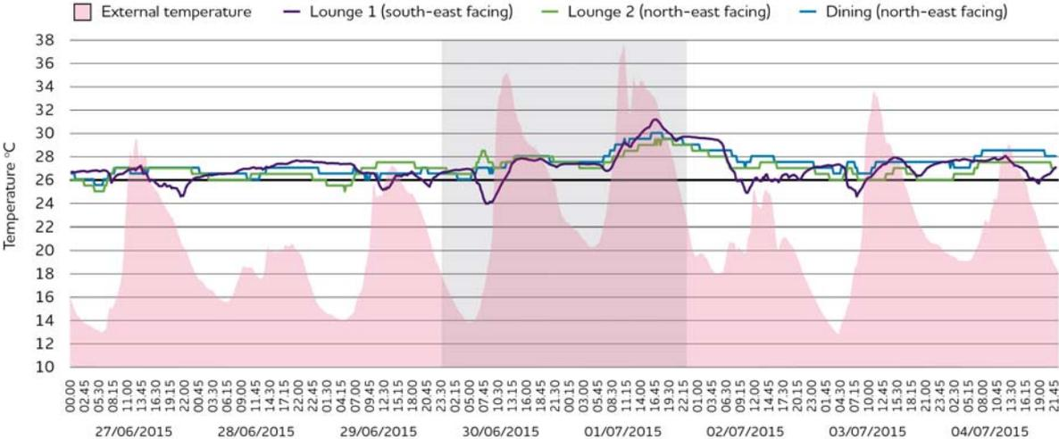
Note: The red dotted horizontal line outlines the threshold temperature for PHE recommended 'cool areas' during a heatwave period.
